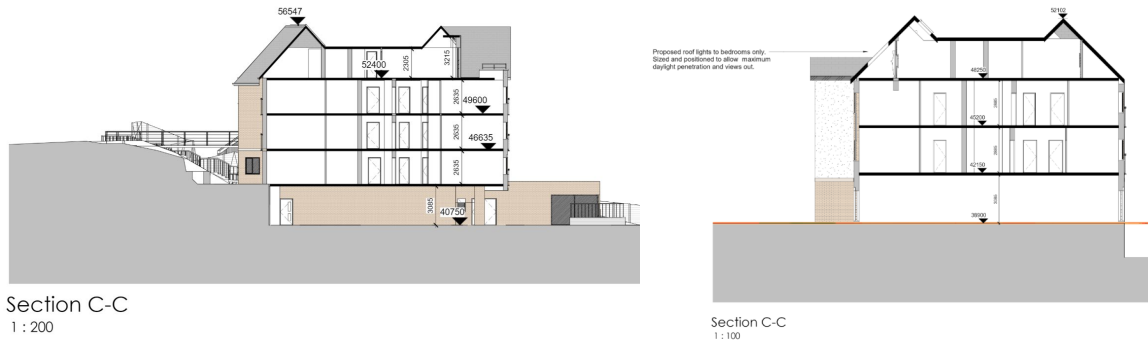
Figure 25 – Sections of Block A (left) and B (right) showing scope for PV panels on flat roof areas set behind roof profiles.
